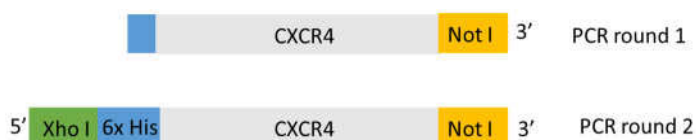
Figure 10 Addition of a 5' His-tag comprising six histidine residues, a 5' Xho I restriction site and a 3' Not I restriction sites in two rounds of PCR. In round 1, part of the His-tag is added to the 5' end of the CXCR4 gene. In round 2, the rest of the tag as well as the Xho I restriction site was added.
