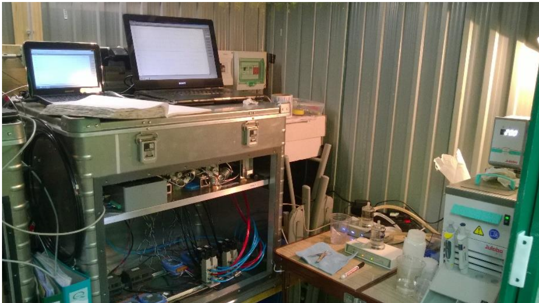
Appendix Figure 16 Two complete oxygen electrode systems for root respiration measurement on F. sylvatica in the instrument hut in situ .
