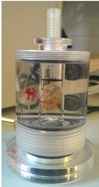
Appendix Figure 13 Root oxygen depletion measurement chamber for Acer platanoides .
