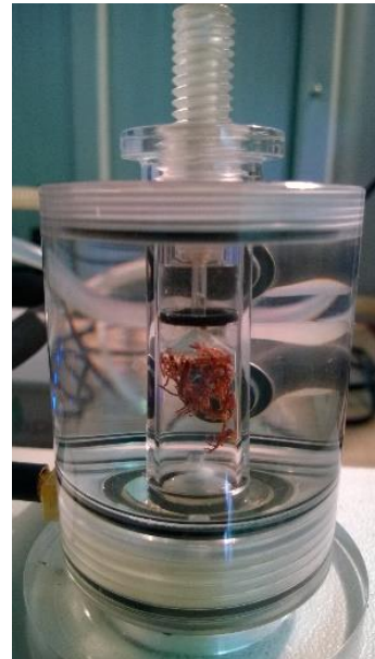
Appendix Figure 14 Root oxygen depletion measurement chamber for Fagus sylvatica .
