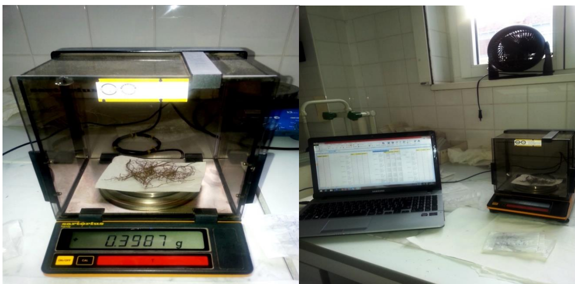
Photo 14: Left; weighing machine till 4 decimal points. Right; recording of sample weights.
