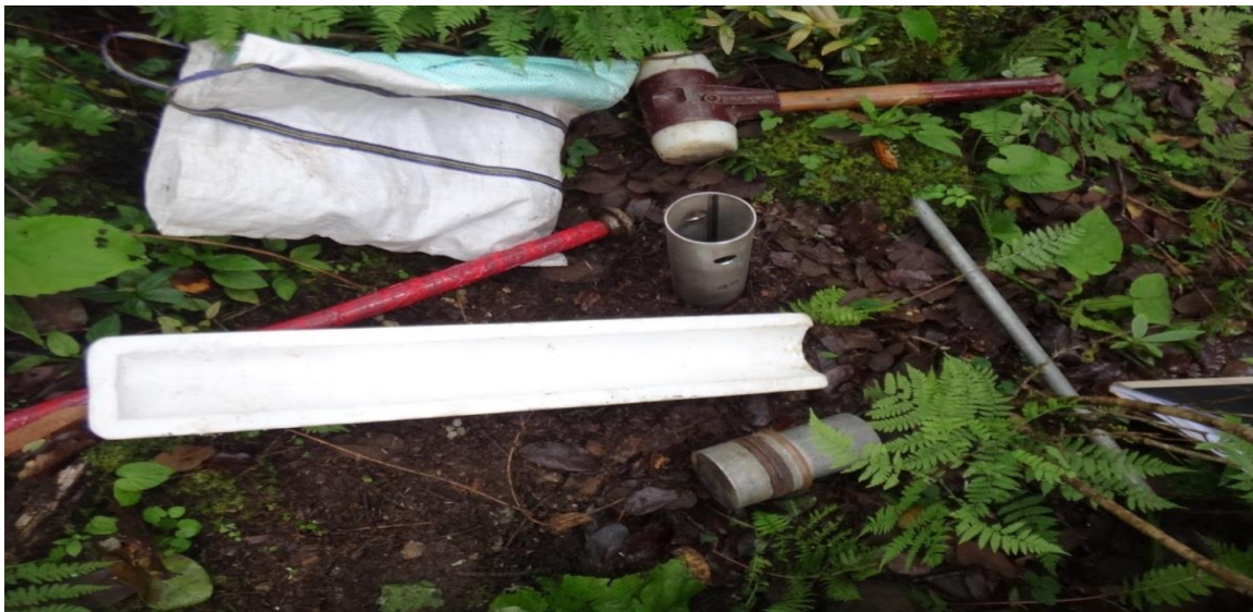
Photo 5: Materials needed for sequential coring; Steel corer, steel rod, Styrofoam tray, plunger, plastic hammer and bag.
