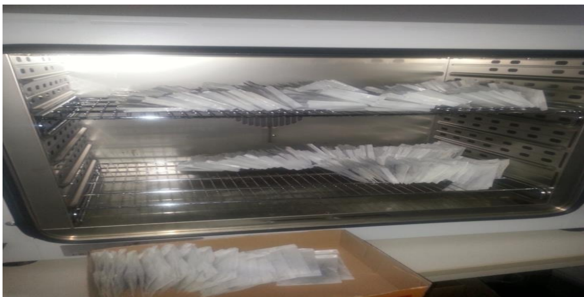
Photo 13: Root samples dried in the oven at 70 0 C for 48 hours.
