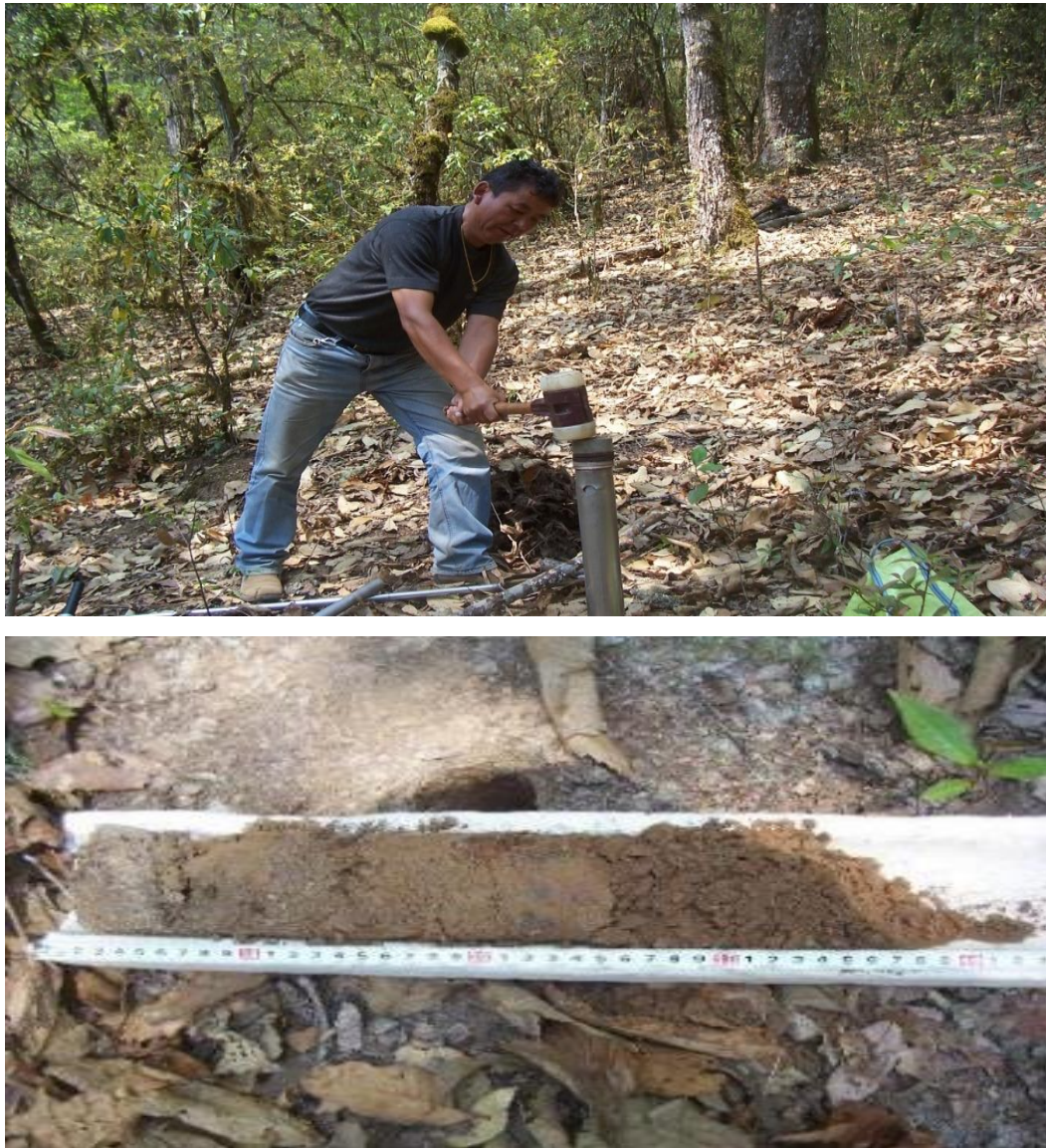
Photo 6: Sequential coring till 30cm depth.
