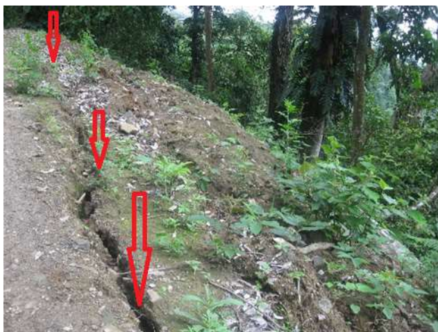
Photo 10: Arc shaped cracks indicating slope failures
