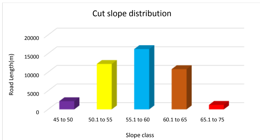
Figure 29: Bar Graph showing cut slope classes and the corresponding road length proportions for farm roads in the watershed
