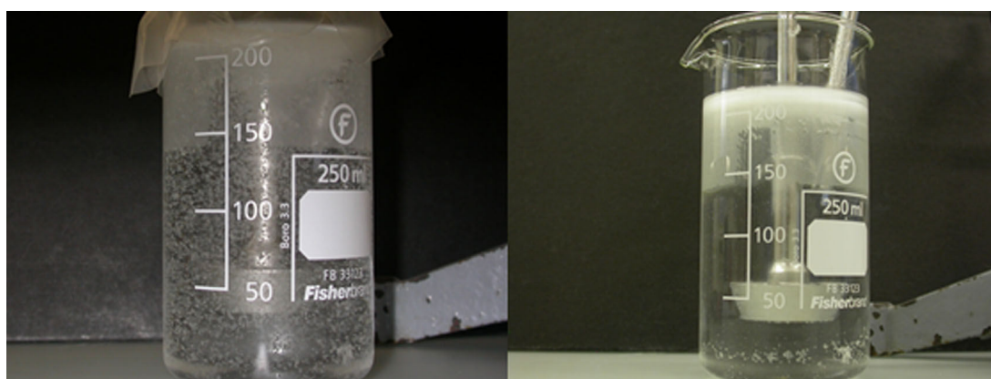
Figure 7. Bulk crystallization in an aqueous two-phase system, stirred (left) and unstirred (right), with phase separation.
