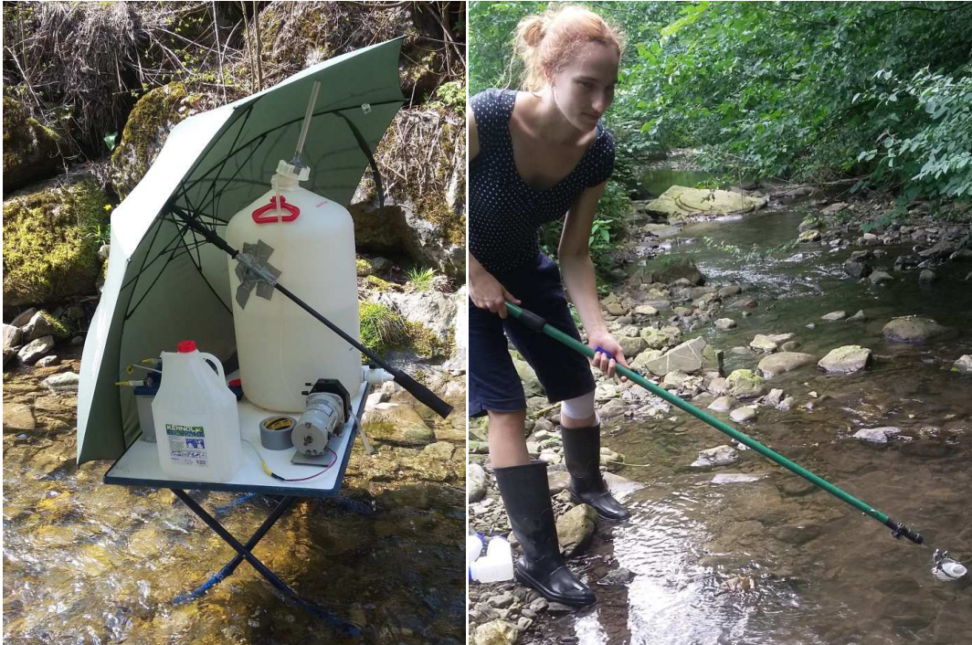
Figure 4: On the left: Nutrient injection device with pump, battery and carboy. On the right: sampling
