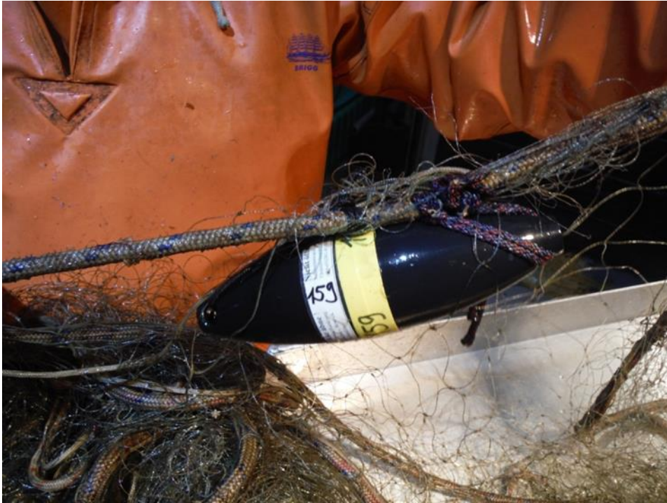
Figure 10: Entanglement of a PAL in meshes. The PAL has been attached in a horizontal position to the floating line of a set net. Due to its tapered ends meshes could be caught resulting in twists which could lead to damages of the net material.
