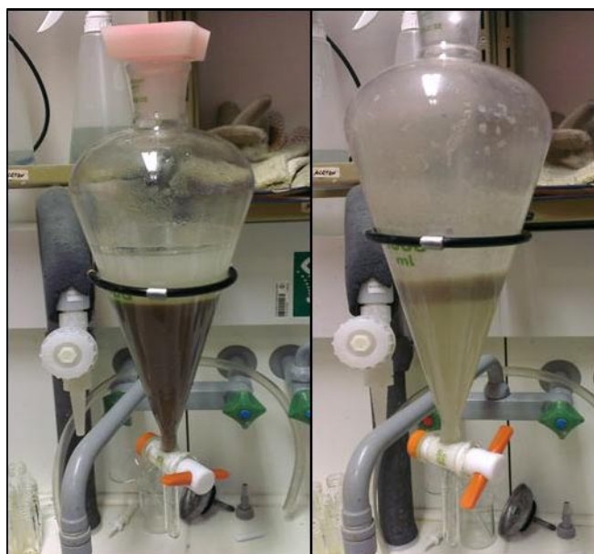
Fig. 32 Separation process by chemical technique before mixing (left side) and after the mixing (right side)
