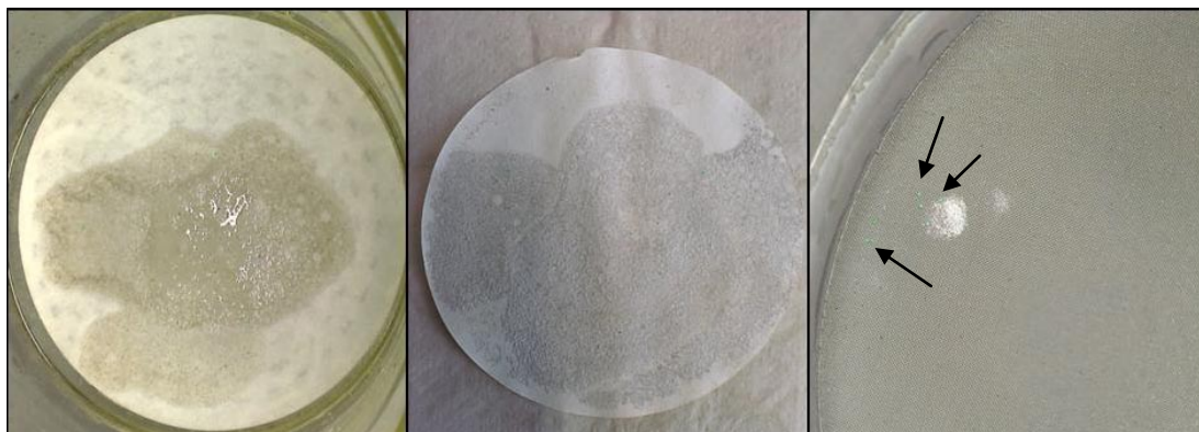
Fig. 33 Isolation process of microplastics in chemical technique: Filtering (left side), drying (middle) and sieving (right side)
