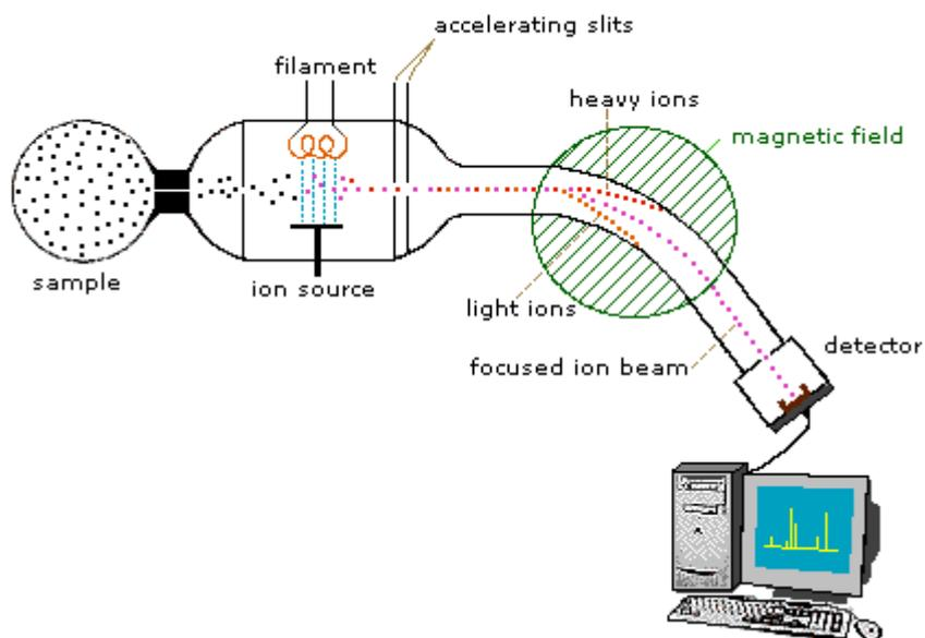
**Figure 3-14 - Schematics of a simple mass spectrometer. The sample is vaporized and ionized. The ionized gas is accelerated and subjected to an electric/magnetic field. The detector counts the abundance of deflected ions with different mass-to-charge ratios.**
