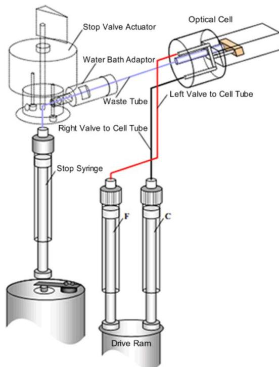
**Figure 3-13 - Schematic layout of a mixing module used in stopped flow apparatus. The drive ram pushes two reagents in syringe F and C into the optical cell. This pushes the old reagents out of the optical cell and fills the stop syringe until the plunger hits the trigger. That stops the drive ram and the start of the data acquisition simultaneously.**
