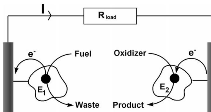
Figure 4: Schematics of an enzymatic biofuel cell: left: enzyme E1 as anodic element, right: enzyme E2 as cathodic element. The combination of both enzymes in an electric cell creates power [Willner et al. 2008]
