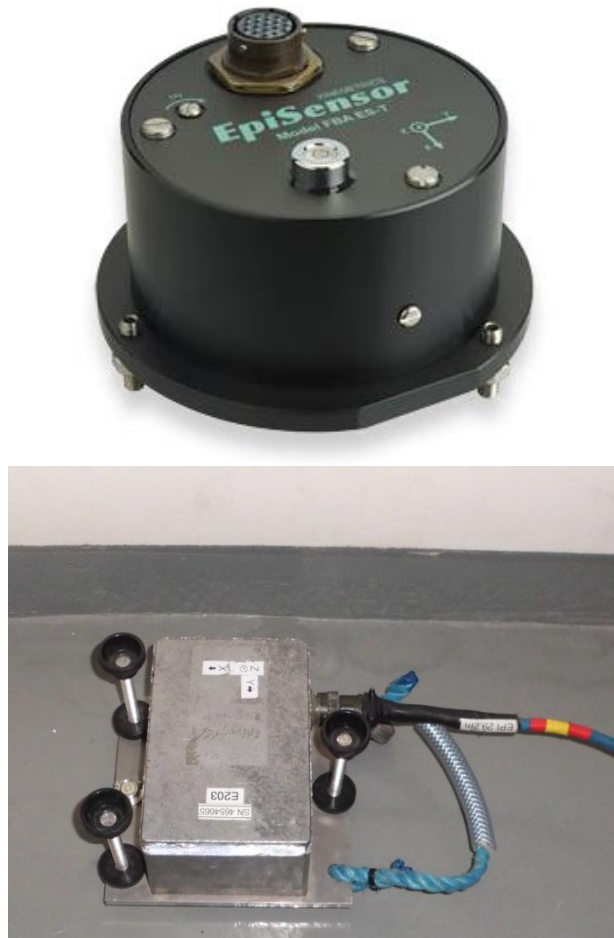
Figure 27: EPI sensor, original housing (TOP), as used (Bottom)
