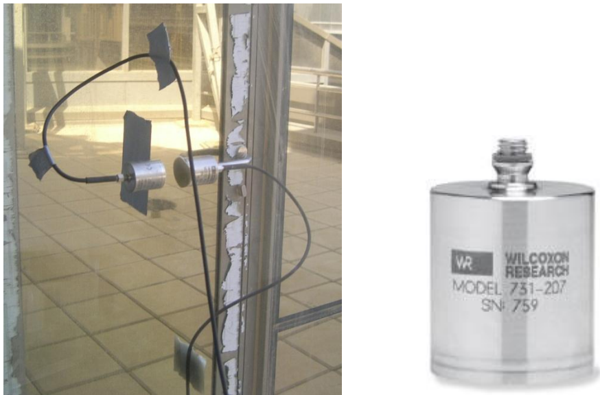
Figure 32: Wilcoxon Model 731-207 (right); Mounting of sensor on glass surface inside and outside (left)
