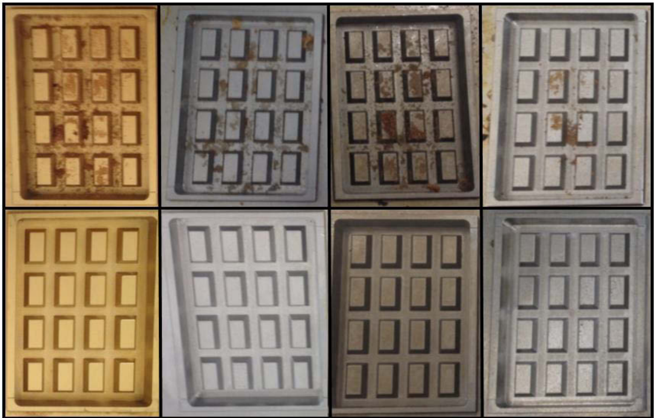
Fig. 1: Baking plates (after baking of waffles from worst ingredient at moderate speed, using Bandex as release agent). From left to right: steel with TiN coating, low alloyed steel, ductile iron, grey iron; – after baking (top row) and after cleaning (bottom row).
