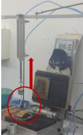
FIGURE 1 Equipment for determination of waffle adhesion force
