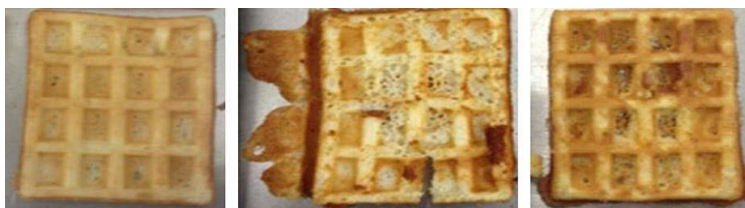
FIGURE 2 Examples for waffles with good and bad quality (from left to right: wheat flour and glycerine (homogenous color distribution and totally filled waffle), rice flour (spotted and broken waffle), wheat flour (spotted, holes, crumble texture)
