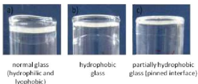
Figure 14: Water covered with a layer of petroleum ether in normal untreated glass (a), in a hydrophobic glass (b) and a glass with a pinned interface (c).
