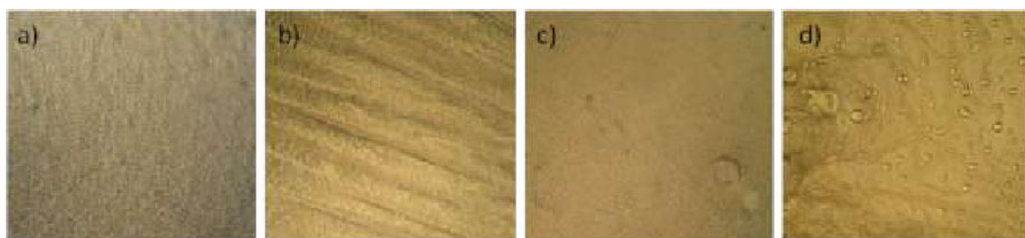
Figure 12: Bright-field microscopy images showing samples directly after pipetting hydrophobic particles, ethanol, petroleum ether, photoinitiator and MMA (a) or tBA (c) into a petroleum ether layer on a water surface. Initially, particles seemed to be homogeneously distributed but after complete solvent evaporation a wrinkled pattern formed b: sample with MMA; d: sample with tBA.
