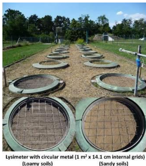
Figure 7: Lysimeters containing loamy and sandy soils fitted with circular metal internal grids for application and sample collection guide.
