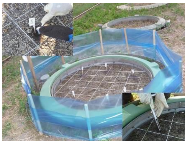
Figure 9: Fencing the lysimeter with plastic sheets after application of veterinary drugs and ^{14}\text{C} -labelled compound.
