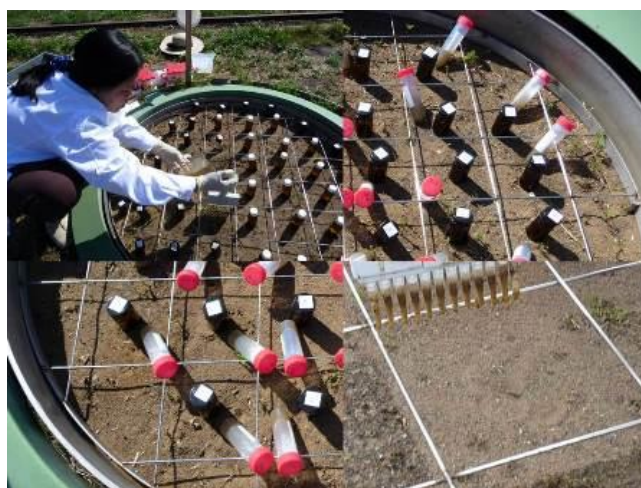
Figure 8: Positioning and application of veterinary pharmaceuticals mixed in cow slurry
