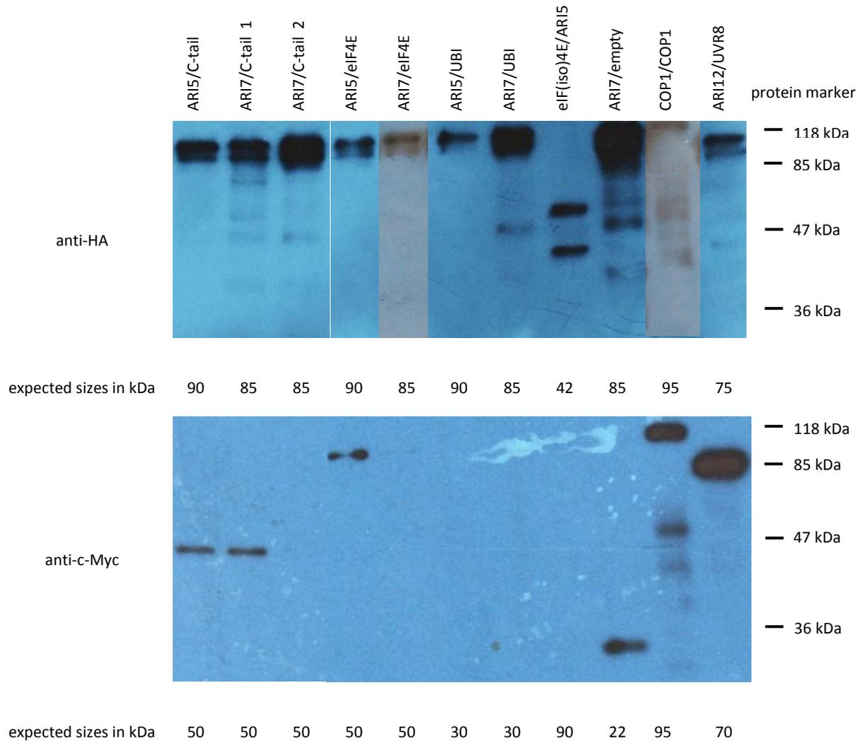
**Figure 25** Western blot 3: At the top 1:1000 rat anti-HA and 1:10000 goat anti-rat HRP; 30 seconds exposure and five minutes for the two extra inserted lanes (grey). At the bottom 1:1000 rabbit anti-C-Myc and 1:7500 goat anti-rabbit HRP; exposure 20 min.
