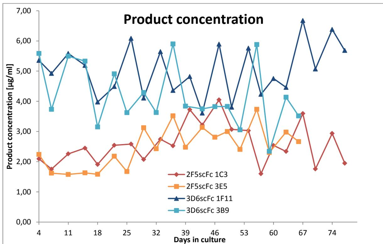
Figure 33: Product concentration over the entire cultivation in the spinner flask.
