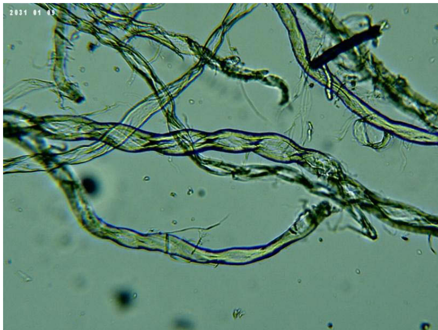
Figure 25. Cotton linters after ultrasonic bath and milling in 18% (w/v) NaOH solution for 20 minutes. (100x BRESSER LCD microscope)
