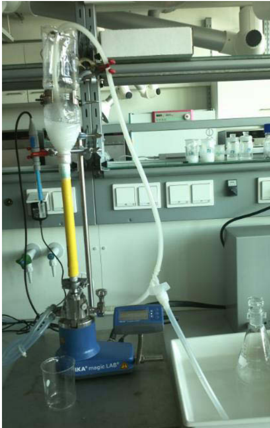
Figure 3. IKA magicLAB MK/MKO colloid mill with cooling water hose and reservoir flask on the top
