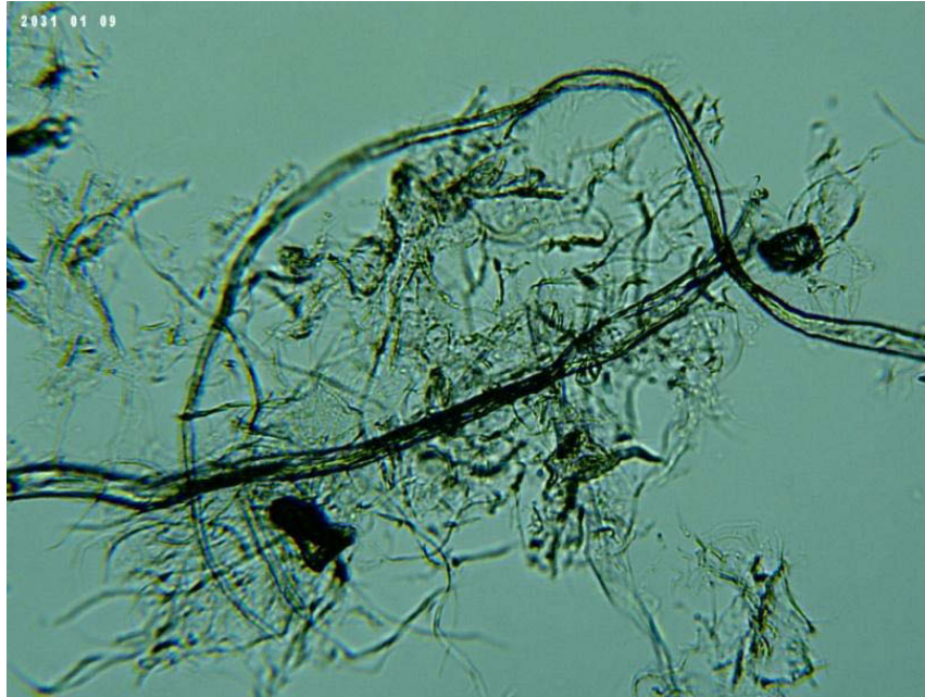
Figure 22. 125 ml DMSO plus 125 ml deionized water (1:1). Pre-swelling and stirring in pure DMSO for 60 minutes, than completion of both mixtures, than milling. 100x (BRESSER LCD microscope)
