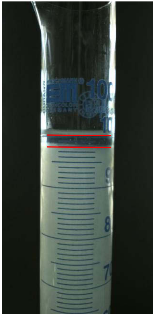
Figure 5. 100 mL graduated cylinder with EMIMAc sample after 10 minutes shows a GS value of 2% after 10 minutes
