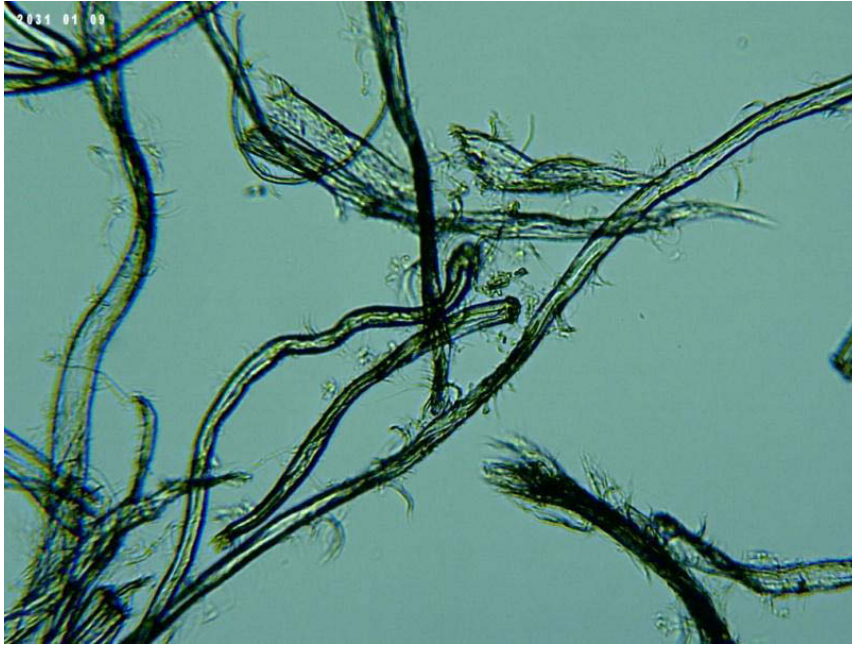
Figure 27. 0.25% cotton linters milled in 0.05 mol/L sodium acetate buffer solution (pH 4.8) + 25 \mu l Celluclast ® (U=600/g cellulose) addition after ultrasonic bath (100x BRESSER LCD microscope)
