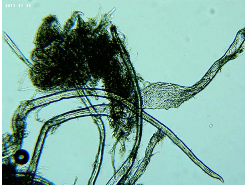
Figure 24. Cotton linters after ultrasonic bath and milling in 10% (w/v) NaOH solution for 20 minutes. (100x BRESSER LCD microscope)
