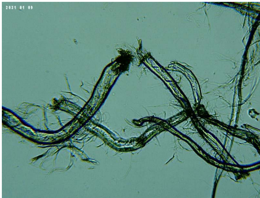
Figure 29. 0.25% cotton linters suspended in 2% aqueous ASA solution (per gram dry cellulose) (100x BRESSER LCD microscope)
