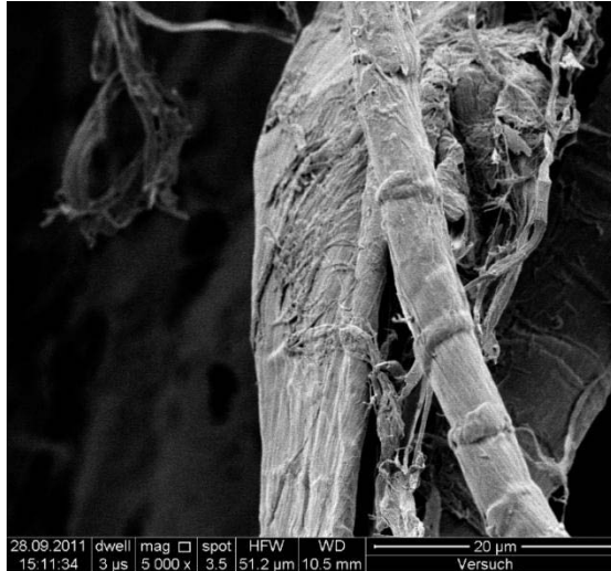
Figure 15. ESEM micrograph of cotton linters after oxidation during milling with 8 mmol/g cellulose NaOCl. PHILPS XL 30 ESEM (5000x)
