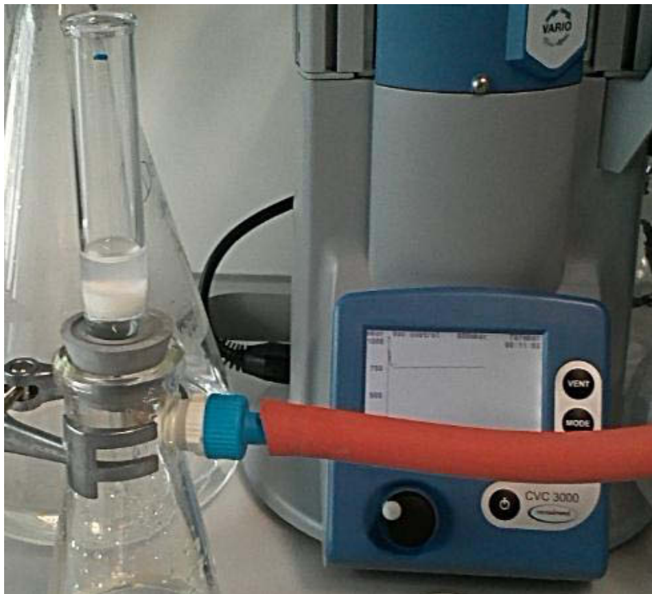
Figure 6. Vacuum flask with class-3 porosity and blue line mark at lower measure point
