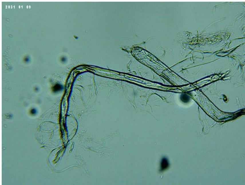
Figure 30. 0.25% cotton linters suspended in 10% (w/w) aqueous CMC solution (100x BRESSER LCD microscope)
