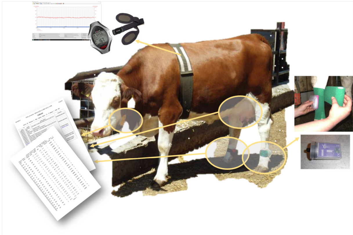
Figure 7: The transparent cow. Girth to hold the electrodes and monitor of the polar ® heart rate measurement system, HOBO ® accelerometer for the automated collection of activity data, pedometer, collar with transponder connecting cow identity with her milk, pedometer and stored life history data.
