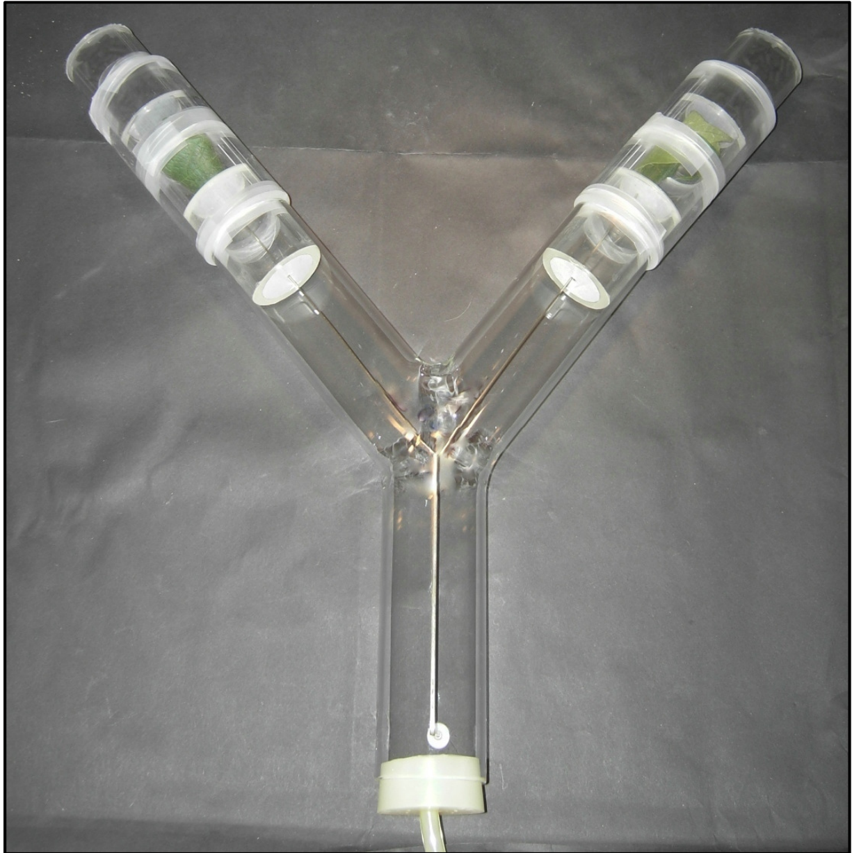
Fig. 4: Y-tube olfactometer used in the experiments (Schausberger et al. 2012).
