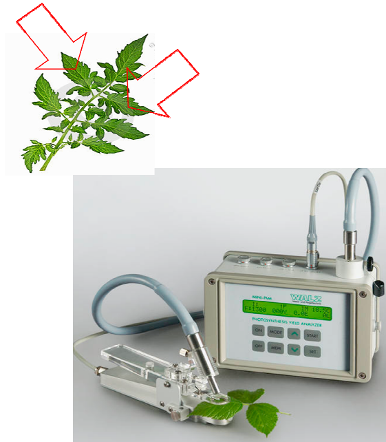
Figure 4: Measuring chlorophyll fluorescence with Mini-PAM
