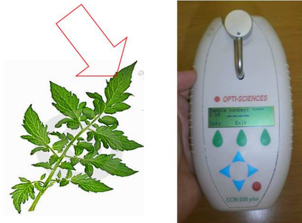
Figure 3: Measuring chlorophyll concentration with CCM 200 plus
