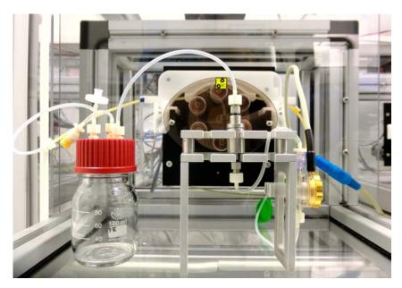
Figure B.4: Image of the bioreactor system stored in the cell culture incubator table
