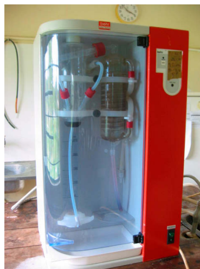
Figure 3.16: Steam distillatory Behr S 1 (behr Labor-Technik GmbH, Düsseldorf, Germany)
