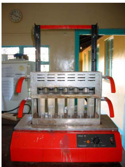
Figure 3.15: Digestion block Behroset InKjel M (behr Labor-Technik GmbH, Düsseldorf, Germany)
