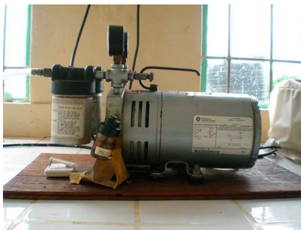
Figure 3.14: Vacuum pump – GE Motors & Industrial Systems, MOD 5KH36KN193HT, 220-250V [source: HEIMBERGER, 2010]
