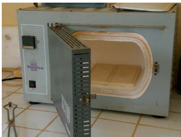
Figure 3.13: Muffle furnace – Barnstead/Thermolyne – 62700 Furnace, Model No F62730, 240V [source: HEIMBERGER, 2010]
