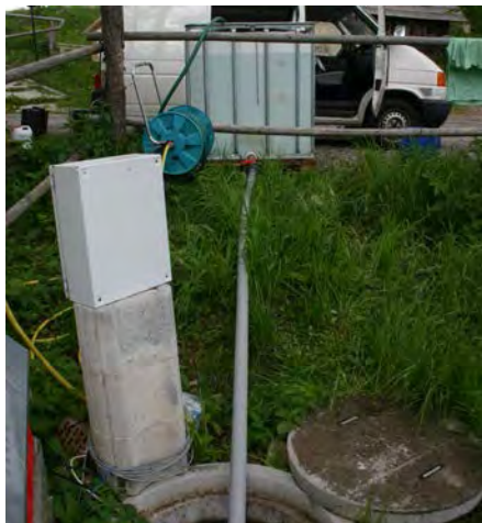
Figure 3-6 Pipe loading the tracer from the tank rapidly into the flexible pipe before FB1
