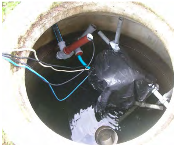
Figure 3-7 Measurement devices for flow (MID underneath black protective plastic cover) and EC (in U-shaped pipe) of effluent FB1
