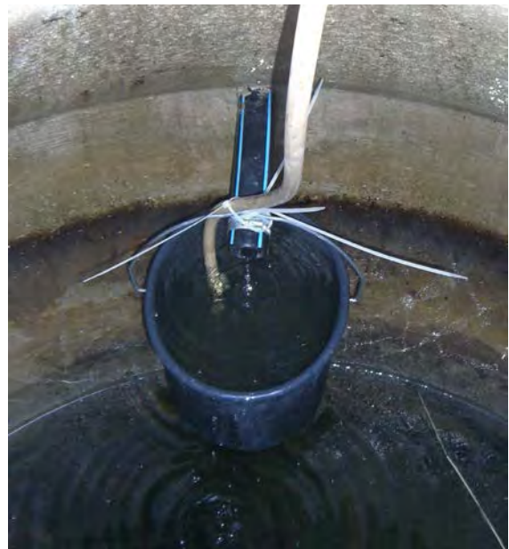
Figure 3-5 Sampling of effluent FB1 from a bucket (white suction hose belongs to automatic sampler)
