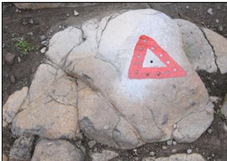
Figure 12: Picture of an GCP in the AM network (Source: Miskas & Molnar, 2010)
