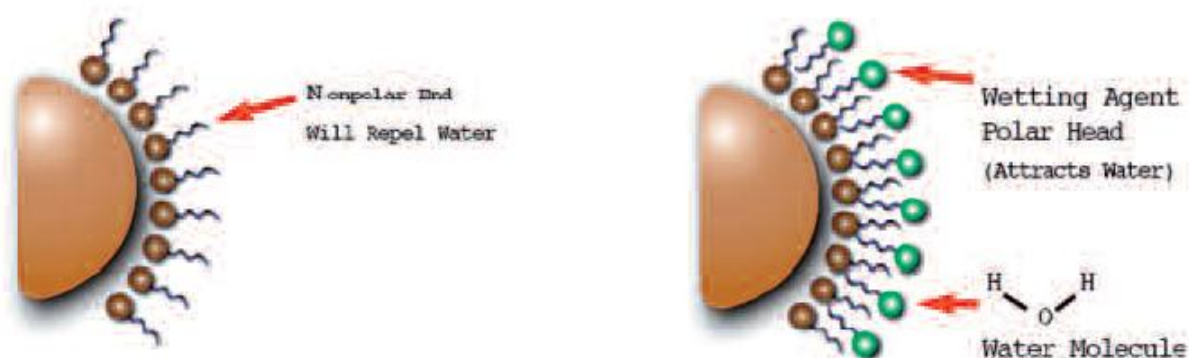
Figure 7: Adsorption of water on hydrophobic material with the help of surfactants (Henle et al., 2007)
