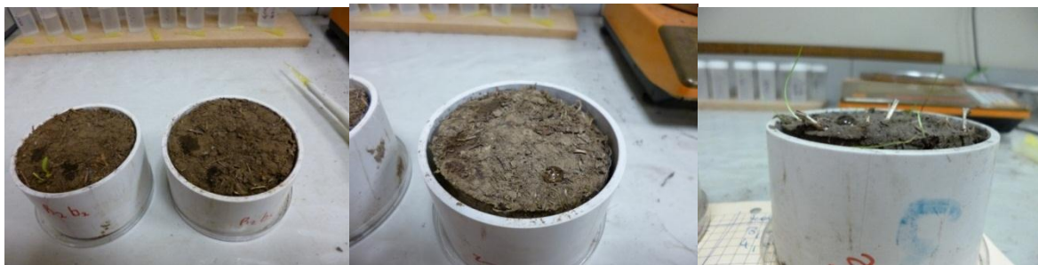
Figure 27: WDPT- test: water droplets testing on soil samples
